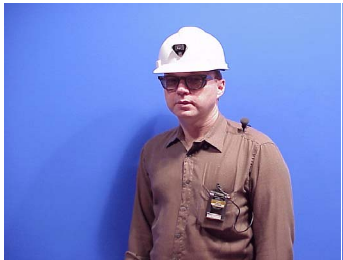
Figure 1. Placement of the dosimeter microphone.
