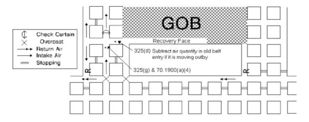
75.325(d) -Quantity for equipment located inby former loading point 75.325(g) -Quantity required to be maintained during removal of longwall equipment 70.1900(a)(4) - Possible sampling location designated by the District Manager
