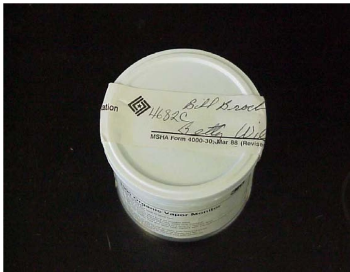
Figure 9- 6. Sealed Passive Monitor Badge Container
