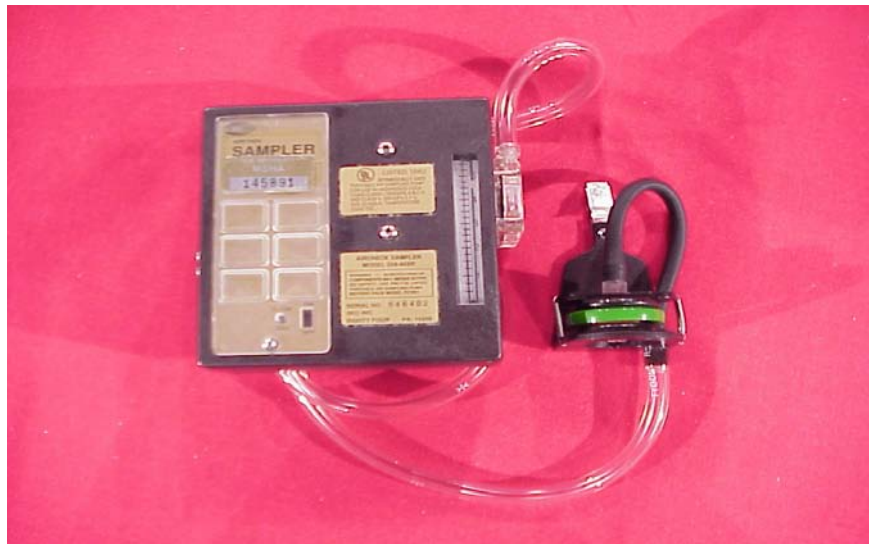
Figure 5- 4. Total Dust Sampling Train
