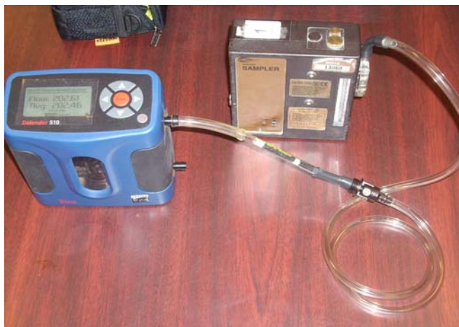
Figure 4C-3-4 Bios Defender 510/SKC Pump with Sorbent Tube Sampling Train Calibration (in-line) Set up.
