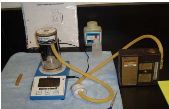
Figure 4C-1-1b. Sensidyne Gilian Gilibrator Set up for Calibration (welding fume MCE cassette/filter in-line)
