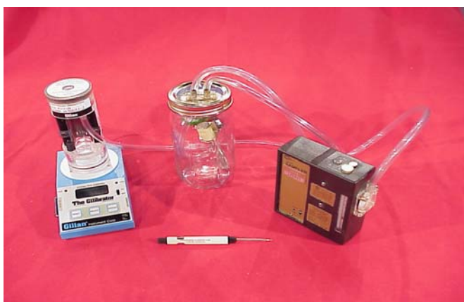
Figure 4C-1-1a. Sensidyne Gilian Gilibrator Set up for Calibration (respirable dust cassette/filter and cyclone in-line inside cal jar)
