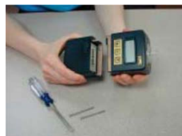
Figure 4A-3-2. SKC AirChek 2000 Battery Pack Removal Step 2.
