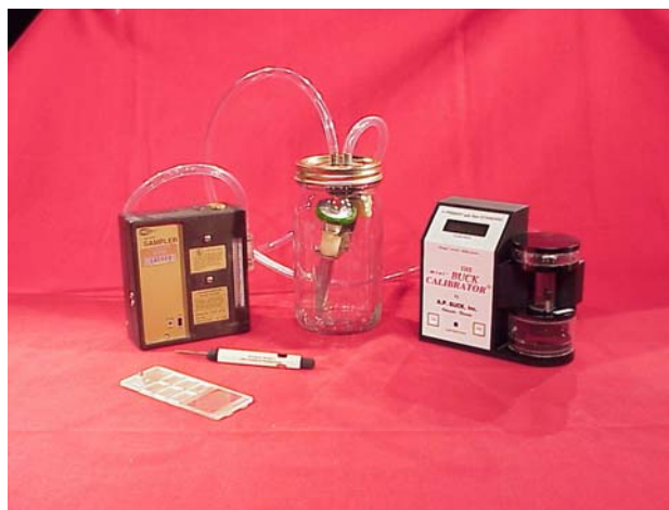
Figure 4C-2-1. mini-BUCK (wet bubble) Sampling Train Calibration Set up.
