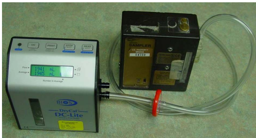
Figure 4C-3-6. Total Dust Cassette In-line Calibration Set up for Bios DryCal DC-Lite.
