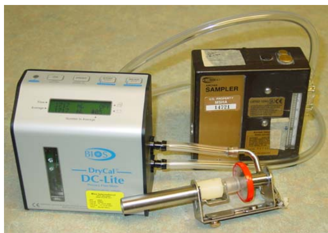
Figure 4C-3-7. Respirable Dust Calibration Set up for Bios DryCal DC-Lite. (Note: NO jar, Not in-line).
