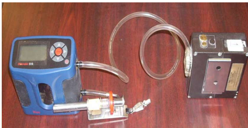
Figure 4C-3-5. Bios Defender 510/ SKC Pump with Respirable Dust Sampling Train Calibration Set up (Note: NO jar, not in-line).
