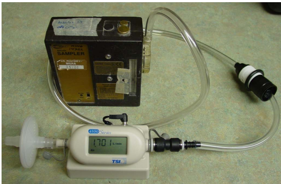
Figure 4C-4-4. TSI Model 4146 Set up for Asbestos Sampling Calibration.
